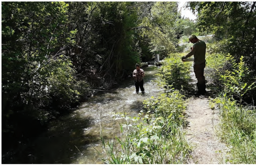
Figure 12. Student field assistants (Madison Groven and Courty Dorn) manually calculated discharge in an acequia (photo by Lily Conrad).
